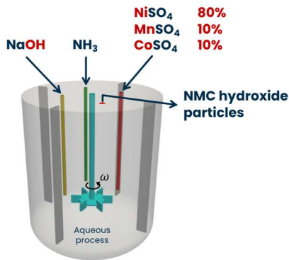
Figure 1: Sketch of the reactive crystallization process.
